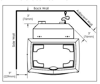
These dimensions are minimum clearances but it is recommended that you ensure sufficient room for servicing, routine cleaning and maintenance.
