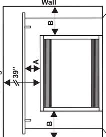
**0" Clearance to combustibles from:** Top, sides, bottom and rear of unit
