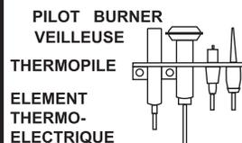
4) Push in control knob all the way and hold in. Continually push and release the black button on spark igniter until pilot lights. Continue to hold the control knob in for about 1/2 minute after the pilot is lit. Release knob and it will pop back up. Pilot should remain lit. If it goes out, repeat steps 1) to 4).
