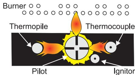
Periodically check the pilot flames. Correct flame pattern has three strong blue flames: 1 flowing around the thermopile, 1 around the thermocouple and 1 flowing across the burner (it does not have to be touching the burner).
