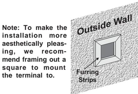
**Note:** If installing termination on a siding covered wall, furring strips must be used to ensure that the termination is not recessed into the siding.
