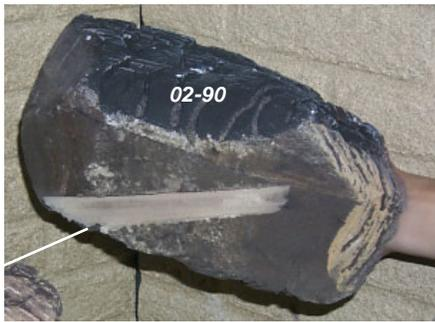
*Cut-out on the underside of the log.*
