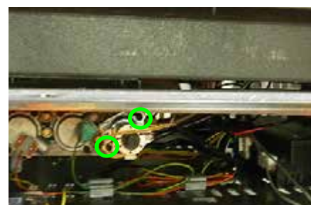
Remove NG Stepper motor and replace with LP Stepper motor
