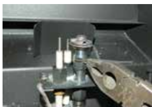
Remove the 2 screws, push Burner Assembly to the left and lift out.
