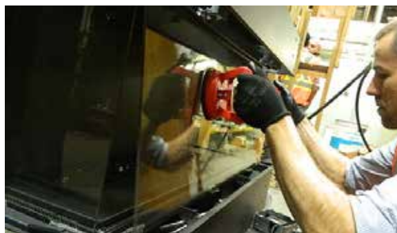
Handle front panel with supplied vacuum clamps
