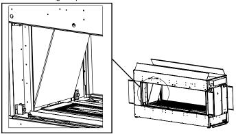
7. Secure side glass by mounting top bracket, then tighten the 2 screws. Repeat steps 5 & 6 on the opposite side.
