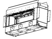
3. Drop the six #3 inner panels into the firebox, then drop the two #2 side covers, as shown below.
