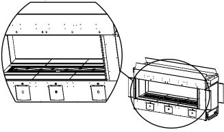
4. Slide in the #4 side panels and secure them by thightening the two screws installed in step 1. Repeat with the #4 side panel on the opposite side.
