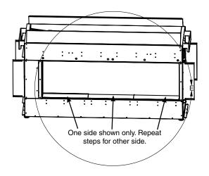
10. Optional: install the glass barrier stopper. If the unit doesn't have a glass stopper, proceed to the next step.
