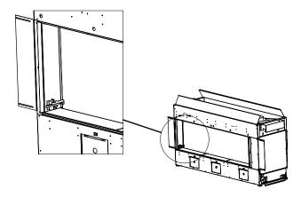
8. Slide the side #5 outer panels between the wall and the barrier stopper bracket. Repeat steps to install the remaining three #5 outer panels using a barrier stop where required.
