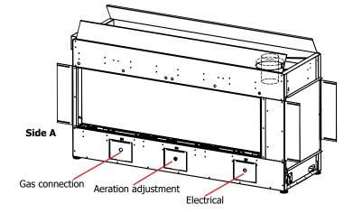
1. Identify the access panel and remove the corresponding outer trim panel by lifting it up and off (centre panel shown opposite).
