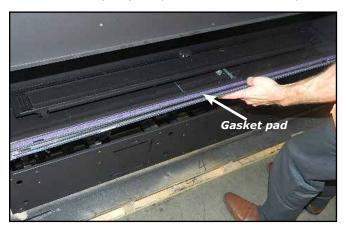
6. Support the glass with one hand and open the 9 lower clamps.
