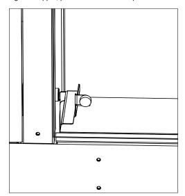
11. Slide the side outer #5 glass panels between the wall and the barrier stopper bracket. If the unit does not have a barrier stopper, stick the side outer panels to the magnets. Repeat steps for the remaining 3 outer sides.
