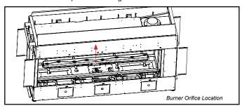
14. Remove the pilot retainer clip with pliers and pull off the pilot cap to expose the pilot orifice.
