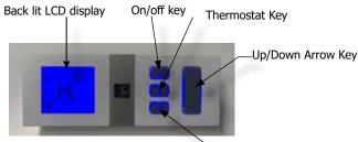
Figure 2: Proflame Transmitter Mode Key
