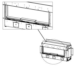
7. Slide the glass barrier stopper in as shown below.
