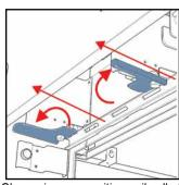
Clamps in open position, rail pulled forward
