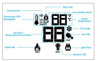
Figure 1: Transmitter LCD Display
