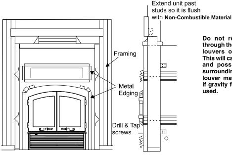
Do not restrict air flow through the top and bottom louvers of the fireplace. This will cause overheating and possible ignition of surrounding materials. Top louver maybe closed only if gravity feed kit option is used.
