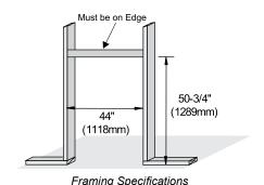
NOTE: Header must be on edge or clearance may not be met to chimney system when installed
