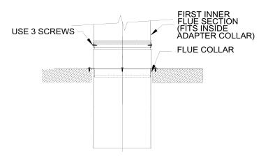
NOTE: For Majestic Flue Pipe, it is recommended that the locking tabs be flattened with pliers to improve the fit into the adapter.
