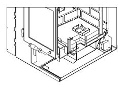
5) Slide the ash drawer shelf into clips on the bottom of the firebox and add thumbscrews to secure in place.
