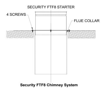
3) Place the first section of flue pipe into the flue adapter collar. Make sure the pipe is seated properly inside the adapter collar and use three (3) #8 self-drilling screws to fasten the pipe to the collar. (Screws provided).
