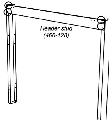
6. Slide the unit into position. Hook up gas, venting, electrical and conversion kit (if purchased) prior to installing the remaining steel studs.
