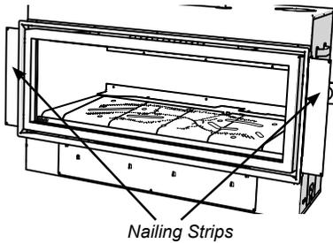
3. Adjust the nailing strips by loosening 2 screws on each nailing strip - adjust and retighten screws.
