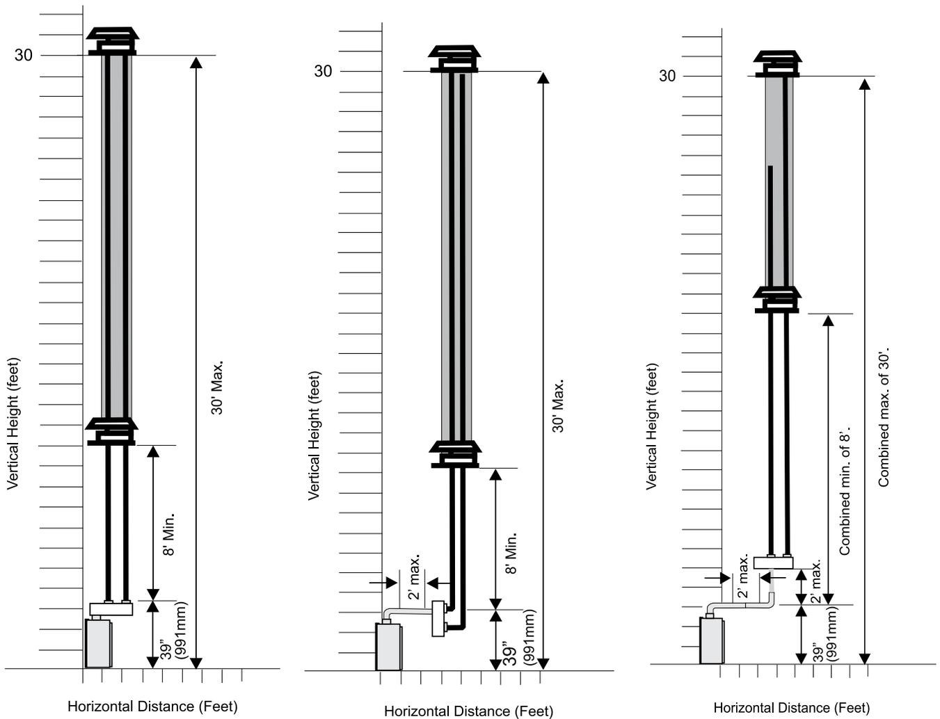
**The shaded area in the diagrams show the allowable vertical terminations.
