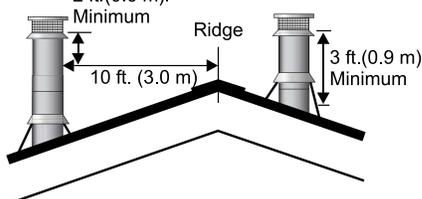
**this minimum level will sometimes help your unit to "breathe" better by allowing a greater draft to be created. This greater draft can decrease problems such as, difficult start-ups, back-smoking when door is open, and dirty glass. It might be sufficient to initially try with the minimum required height, and then if problems do arise add additional height at a later date.**
