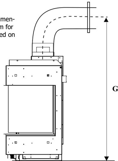
\* The framing depth does not take into account plasterboard/timber or similar materials against the back wall. The framing depth will need to change based on the thickness of the materials (example: C - 483 mm framing depth + 13 mm plasterboard = 496 mm).
