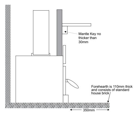
NOTE: If using 24mm cement sheet the hearth will need to be extended to 570mm.
