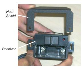
Secure Heat Shield onto Receiver with 2 x #10 x 1/2" screws. Ensure the bottom of the Heat Shield is flush with the Receiver as shown in the diagram below.
