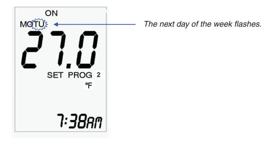
Once the programs have been copied over to the other days of the week, the Remote Control will automatically return to normal Program mode after the last button is released, after approximately 20 seconds.
