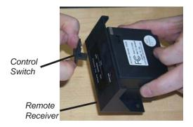
2) Remove spring loaded Battery Pack by pushing in and then pulling out.
