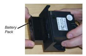
3) Remove Receiver from Bracket and discard bracket. (This Bracket is no longer required after this step.)
