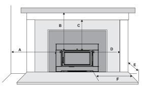
Minimum Hearth Extension for the front (E) and sides (F) are measured from the fuel door opening.
