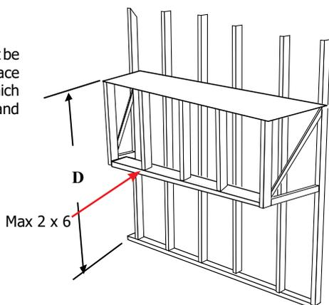
**Note: Unit must be installed onto a solid backwall - do not install directly onto studs.**
