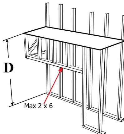
**Note: Unit must be installed onto a solid back wall - do not install directly onto studs.**
