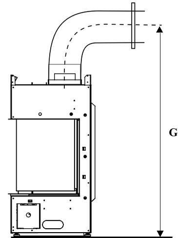
Note: This appliance must be installed on a level and solid surface such as a plywood floor which must be the full width and depth of the appliance.
