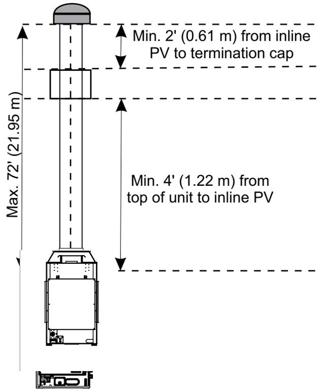
Max. of 72' (21.95 m), using up to six 90° elbows
