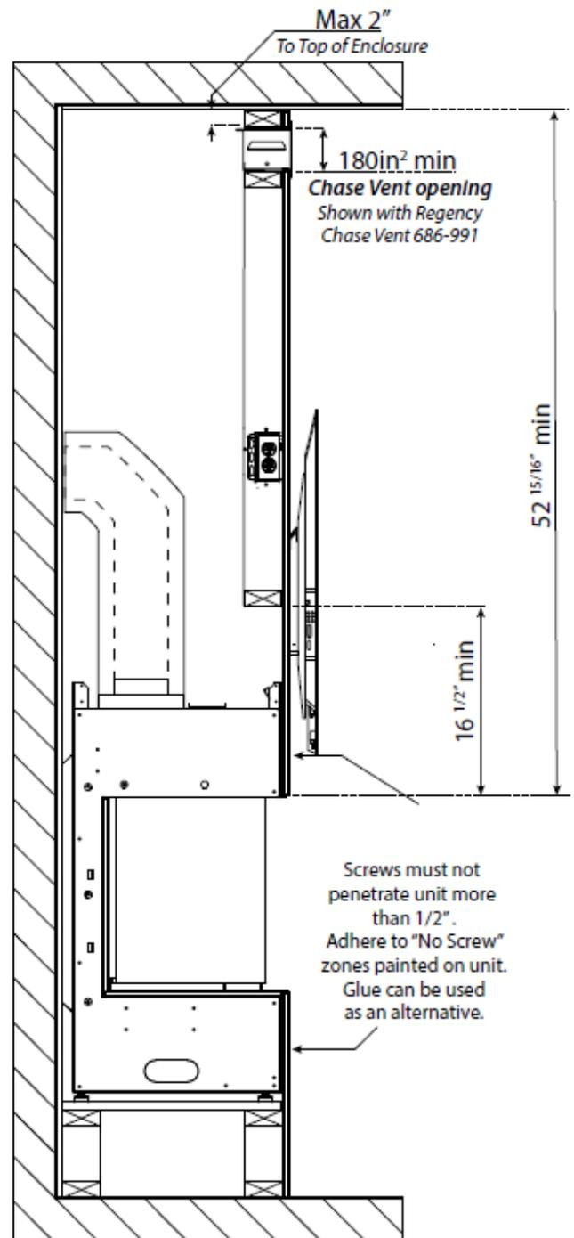
Note: The TV mounting bracket cannot be secured directly to the appliance. It must be secured to framing. The TV depicted in the picture may need to be higher depending on the style of TV mounting bracket used.
