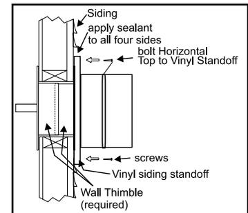
replaced with appropriate fasteners for stucco, brick, concrete, or other types of sidings.
