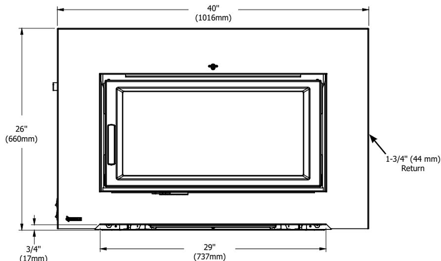
**DIMENSIONS - STANDARD CAST FACEPLATE AND OFFSET FLUE COLLAR - HI500-1**
