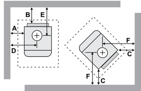
**NOTE:** This clearance is also required for air space between the appliance and wall/ceiling. Clearances to combustibles are for the safety of the property. To avoid overheating and damaging the appliance these clearances should be maintained for non-combustibles also.
