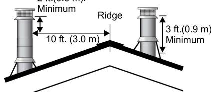
support to a minimum height of 3 feet above the roof penetration, or 2 feet above any point within 10 feet measured horizontally. There must be at least 3 feet of chimney above the roof level.
