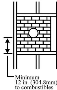
Minimum chimney clearance to brick and combustibles 2 in. (50.8 mm)
