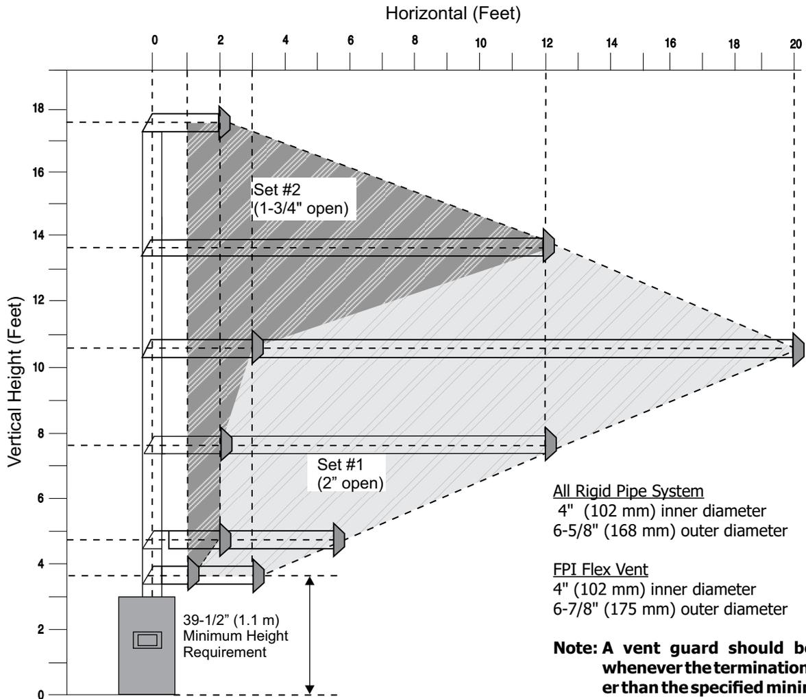
**Note: A vent guard should be used whenever the termination is lower than the specified minimum or as per local codes.**
