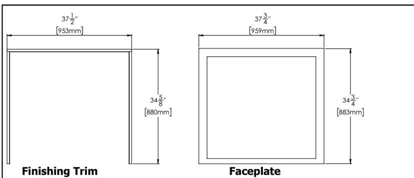
Note: Gas connection is from the left hand side of the appliance & electrical connection on right hand side of the appliance. A metal receptacle box is supplied/installed with the appliance to make all 120 volt electrical connections.
