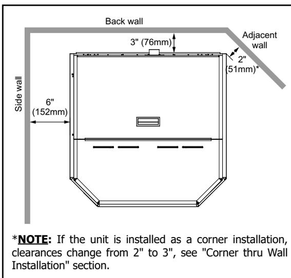
**\*NOTE:** If the unit is installed as a corner installation, clearances change from 2" to 3", see "Corner thru Wall Installation" section.
