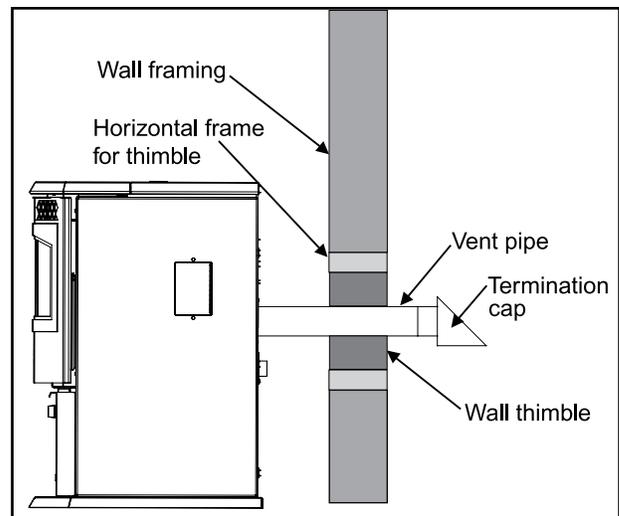
*Straight through Wall Installation - Side View*
