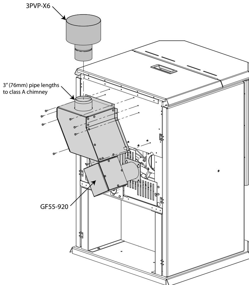
\*In order to achieve the maximum rated efficiency of 75% HHV purchase of a top vent adaptor kit (GF55-920) is required. Use the sheet metal screws provided to attach the kit to the rear of the unit as shown. Please see kit instruction manual for more detailed installation instructions.
