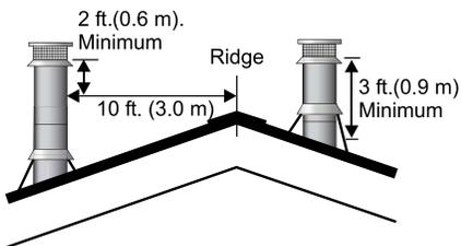
**Note:** Increasing the chimney height above this minimum level will sometimes help your unit to "breathe" better by allowing a greater draft to be created. This greater draft can decrease problems such as, difficult start-ups, back-smoking when door is open, and dirty glass. It might be sufficient to initially try with the minimum required height, and then if problems do arise add additional height at a later date.
