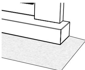
**Note:** All non-combustible facing material should butt up cleanly to the flanges around the firebox opening.
