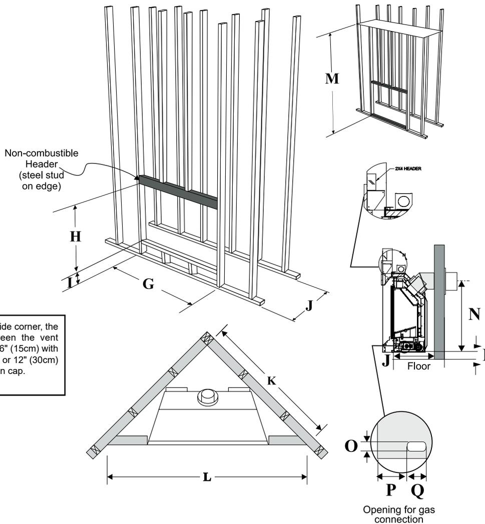
**NOTE:** If this is an outside corner, the minimum distance between the vent and the outside corner is 6" (15cm) with AstroCap termination cap or 12" (30cm) with Rigid Vent termination cap. (For example Dura-Vent)
