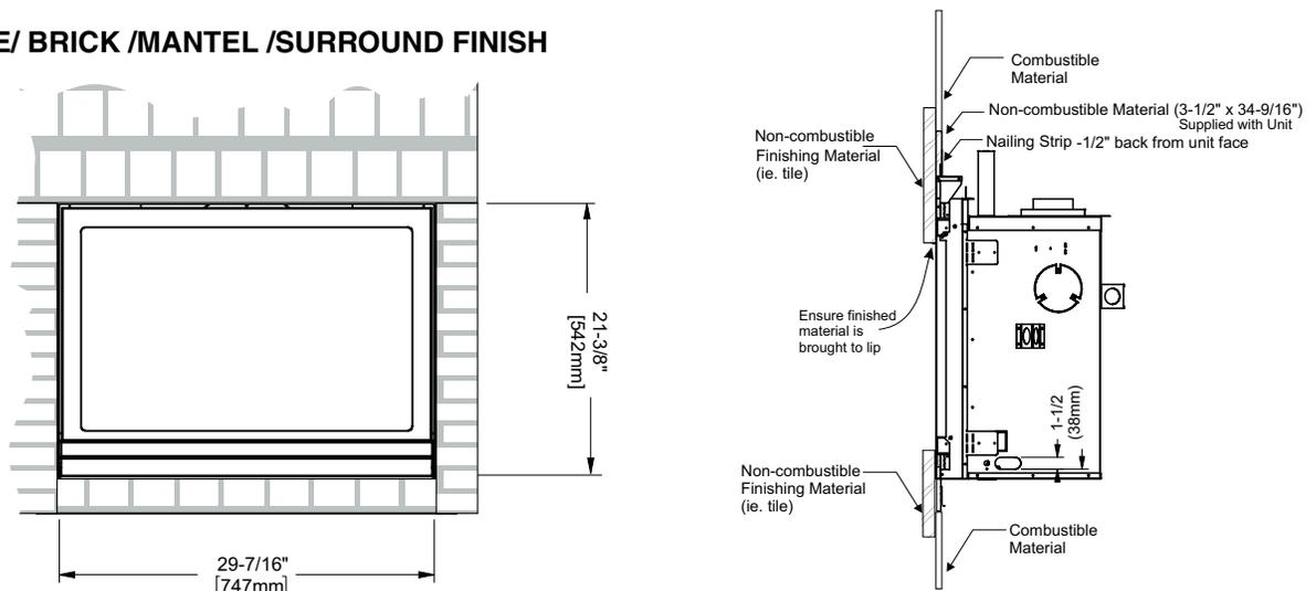
6. If applying a non-combustible facing it may be installed over the metal surface of the firebox of the unit in the area shown below.
