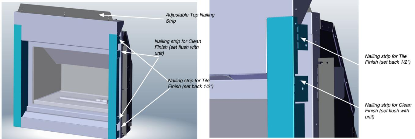
1. Frame in the enclosure for the unit with framing material.
