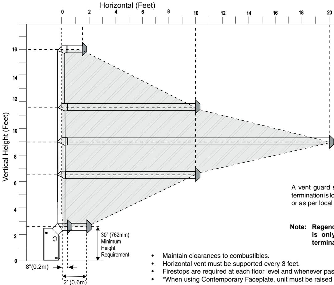
A vent guard should be used whenever the termination is lower than the specified minimum or as per local codes.
