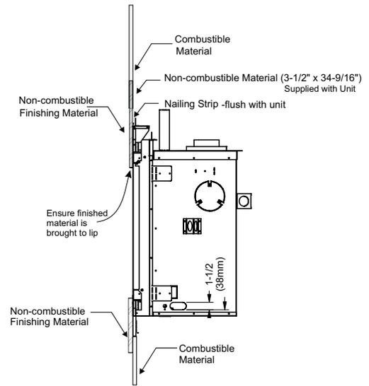
**NOTE:** The 3-1/2" x 34-9/16" non combustible material supplied with this unit can be replaced if trying to achieve a clean finish. A large piece of non combustible material (ie. 4' x 8' x 1/2") can be used to eliminate taped seams on or near unit.
