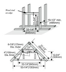
\*\*\* **NOTE:** If using the optional Vignette finishing trim, this can be installed as a 3-sided or 4 sided finish trim. If choosing to use this as a 4 sided finish trim the framing would need to be increased in height by  $1-1/4^{"}$  inches minimum in order for this to fit. This must be to the finished floor. (Example:  $34 3/4^{"}$  framing height +  $1-1/4^{"}$  to bottom of 4-sided finishing trim +1/2 thick finished floor =  $36 1/2^{"}$  total framing height
