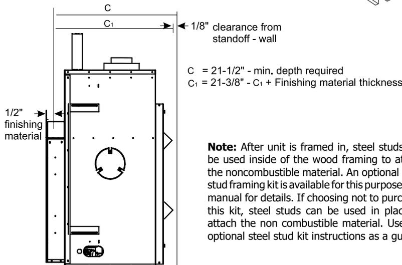
**Note:** After unit is framed in, steel studs can be used inside of the wood framing to attach the noncombustible material. An optional steel stud framing kit is available for this purpose—see manual for details. If choosing not to purchase this kit, steel studs can be used in place to attach the noncombustible material. Use the optional steel stud kit instructions as a guide.
