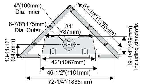
3. For exterior walls, insulate the enclosure to the same degree as the rest of the house, apply vapour barrier and drywall, as per local installation codes. **(Do not insulate the fireplace itself.)**
