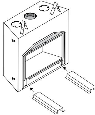
**Install Top Standoffs & Side Nailing Strips before unit is slipped into position. See the "Unit Assembly Prior to Installation" section for assembly details.**
