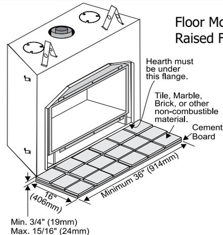
No hearth is required when the unit is raised 3" (76mm) off of the floor surface
