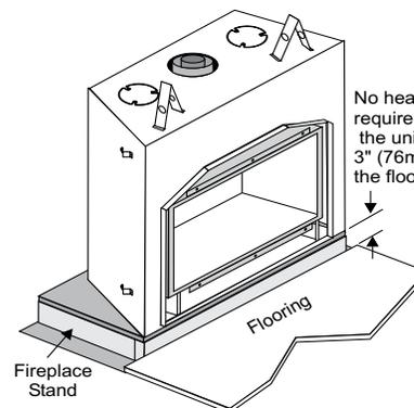
You must take into account the depth of the floor covering (carpet, tile, linoleum, etc.) when determining the height of the fireplace stand.
