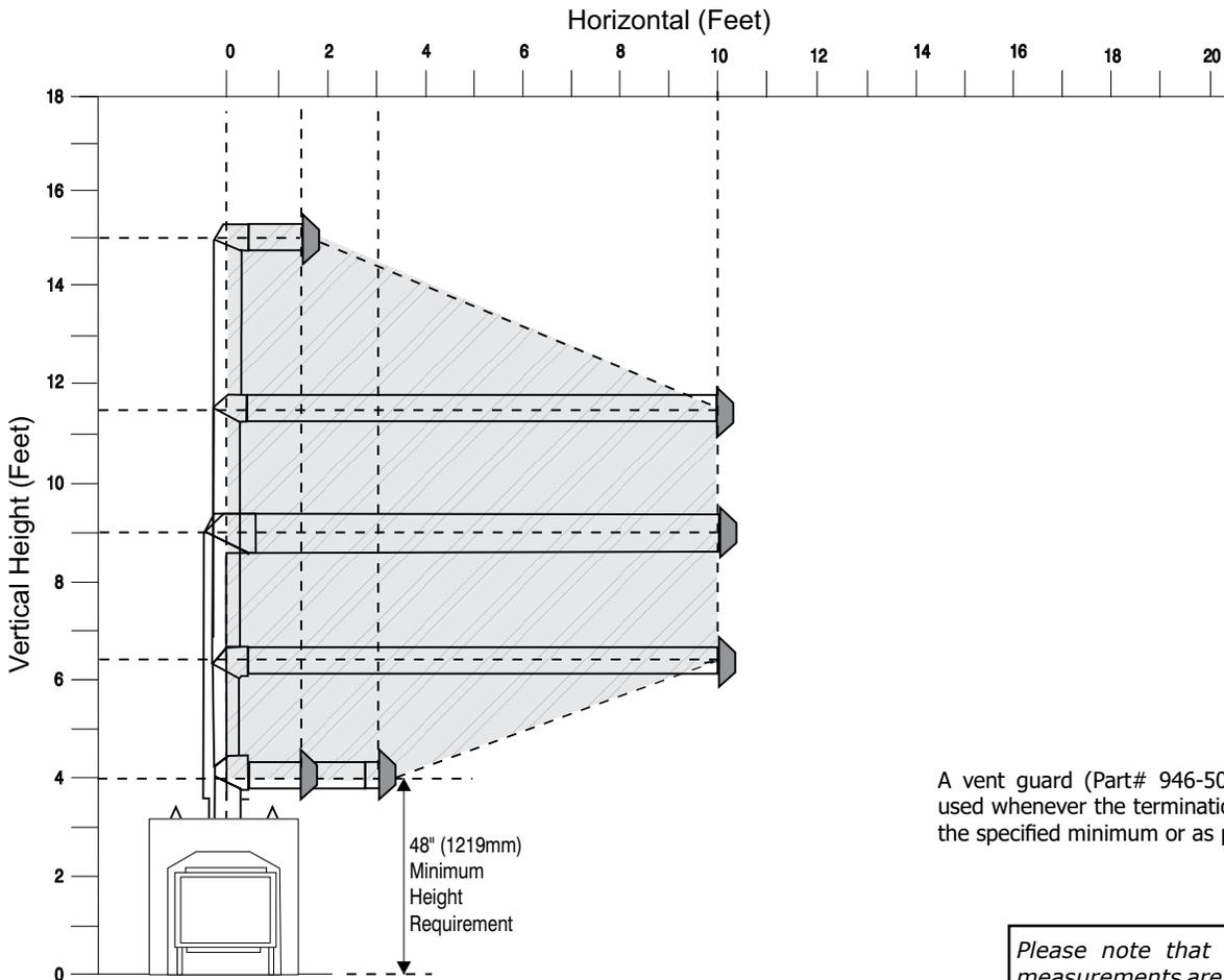
A vent guard (Part# 946-506/P) should be used whenever the termination is lower than the specified minimum or as per local codes.
