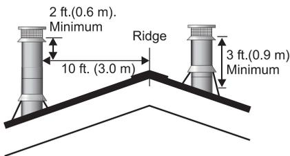
**Note:** Increasing the chimney height above this minimum level will sometimes help your unit to “breathe” better by allowing a greater draft to be created. This greater draft can decrease problems such as, difficult start-ups, back-smoking when door is open, and dirty glass. It might be sufficient to initially try with the minimum required height, and then if problems do arise add additional height at a later date.
