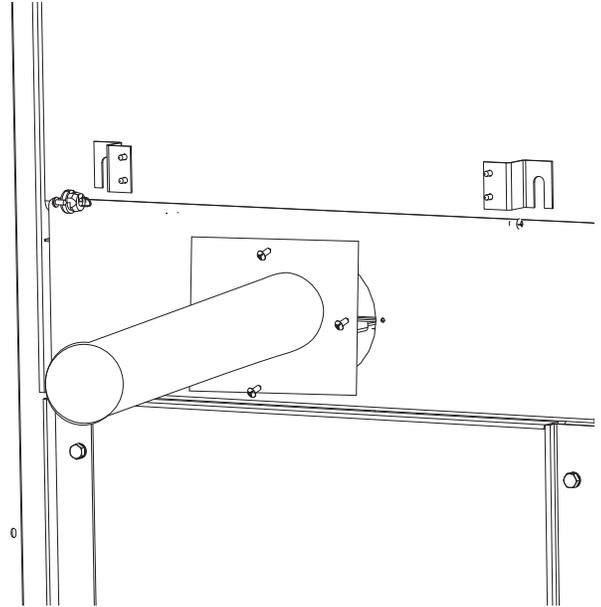
3) Reinstall the backing plate over the air kit pipe. Secure with 4 screws removed from step 1.
