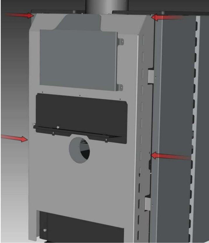
2) Center the plate / pipe over the opening on the back of the stove. Secure with 4 self tapping screws.
