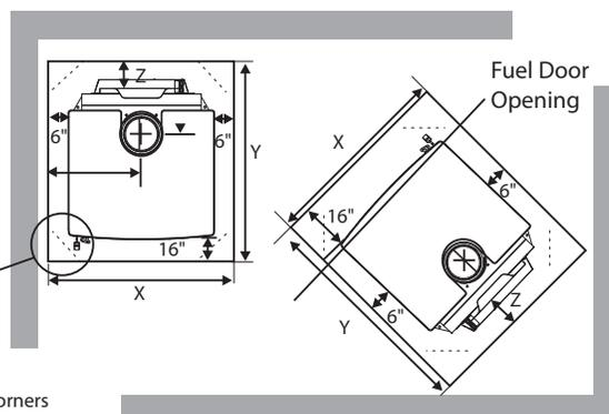
**Note:** If venting horizontally, floor protection must extend under the chimney connector and 2" inches beyond each side.
