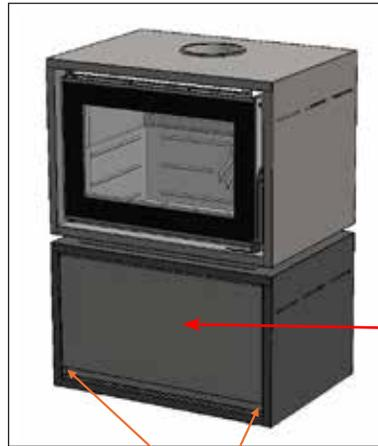
Transit screws to keep stacker door closed – remove to access storage area
