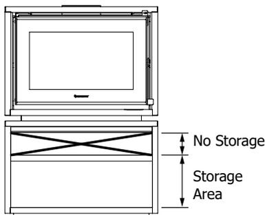
**WARNING: DO NOT PLACE WOOD OR ANY OTHER COMBUSTIBLE MATERIALS ABOVE THE BASE OF THE FAN AIR INLET.**
