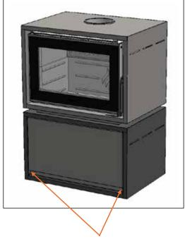
Transit screws to keep stacker door closed – remove to access storage area
