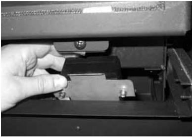
*DC Spark Box mounting plate partially removed.*
