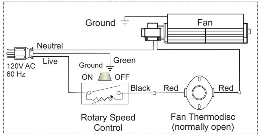
NOTE: Wiring schematics for P36E-4 (120 Volts), plug-in fan circuit with speed control switch on wall.
