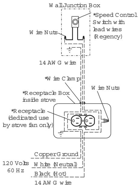
P36 Electrical Connection Alternative Scheme "B", Power at Switch
