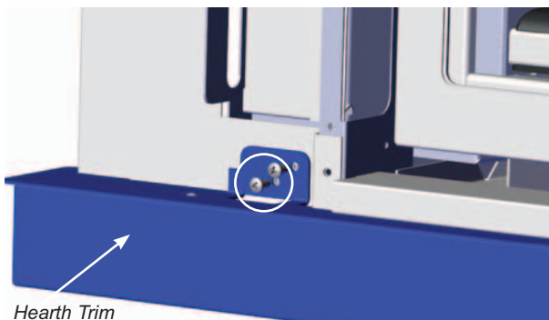
Diagram 3—Hearth Trim Secured to Backing Plate
