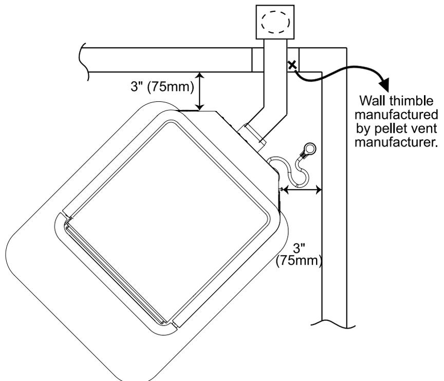
Figure 9: Corner Installation
