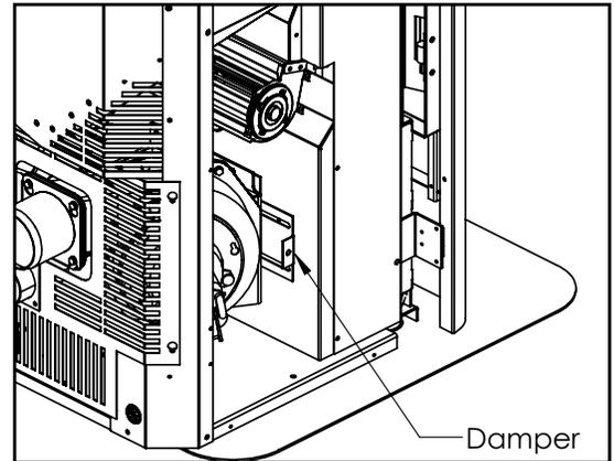
Figure 29: Slider/Damper Adjustment
