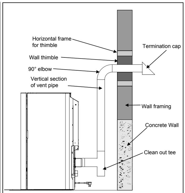
Figure 13: Venting with Concrete Wall Behind Unit
