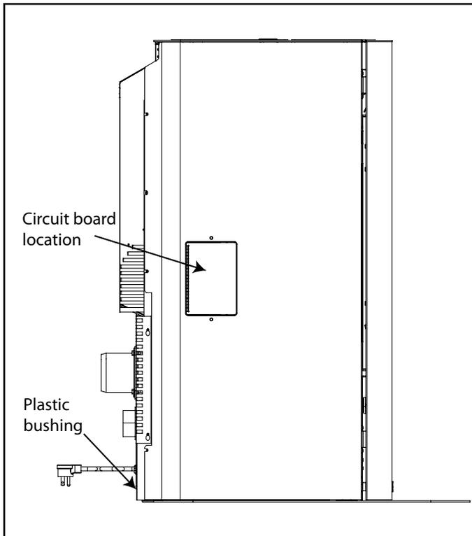
Figure 26a: Circuit Board Location
