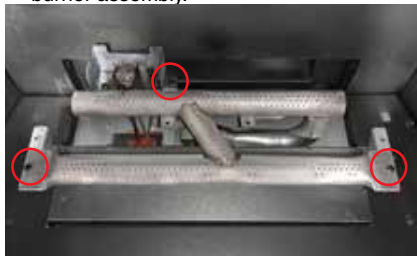
Diagram 2: Slide burner assembly to the right—then remove.
