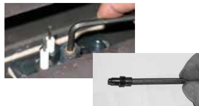
Diagram 2: Slide burner assembly to the right—then remove.
