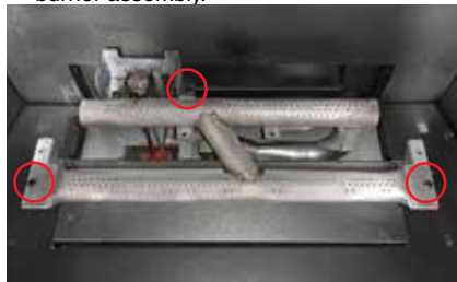
Diagram 2: Slide burner assembly to the right—then remove.
