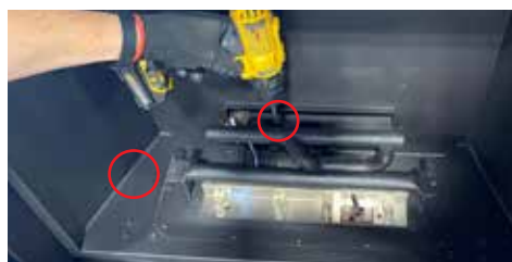
Diagram 2: Slide burner assembly to the right—then remove.
