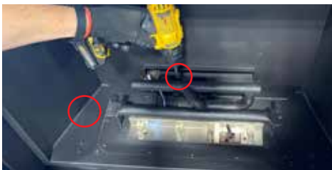
Diagram 2: Slide burner assembly to the right—then remove.
