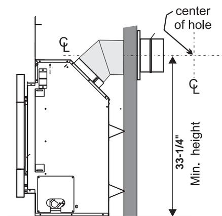
**IMPORTANT:** Do not locate termination hood where excessive snow or ice buildup may occur. Be sure to check vent termination area after snow falls, and clear to prevent accidental blockage of venting system. When using snow blowers, make sure snow is not directed towards vent termination area.
