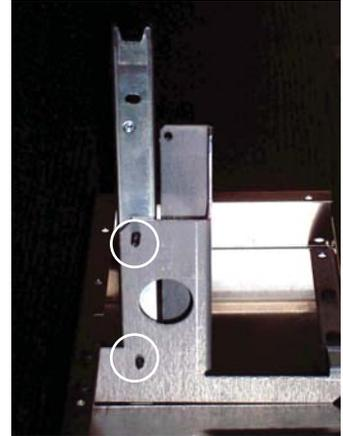
10) With brackets and inner slides attached to the lower faceplate panel - guide the lower faceplate panel into the outer slides located in the bottom part of the unit. See inset. Push in until flush with upper faceplate.
