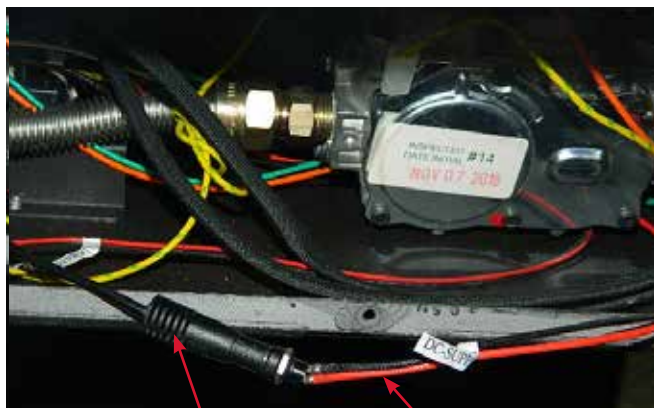
DC supply wire from wiring harness
