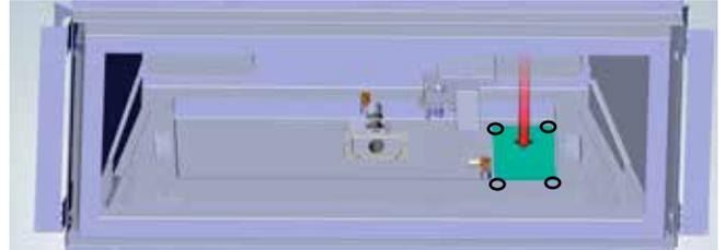
7. Remove valve tray by removing twelve (12) screws in locations shown in Diagram 4.
