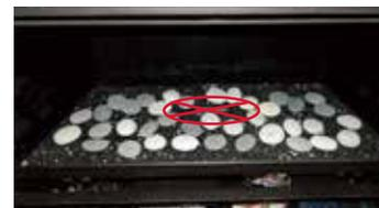
**NOTE:** Volcanic Stones are **NOT** to be placed anywhere on the burner ports or Pilot assembly area.
