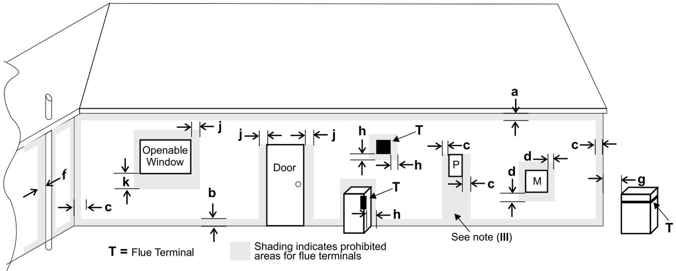
**Minimum clearances required for balanced flue terminals or the flue terminals of outdoor appliances according to AS5601-2004 (AGA gas installation code) or NZS5262 / NZS5266 (New Zealand) and local authorities having jurisdiction.**
