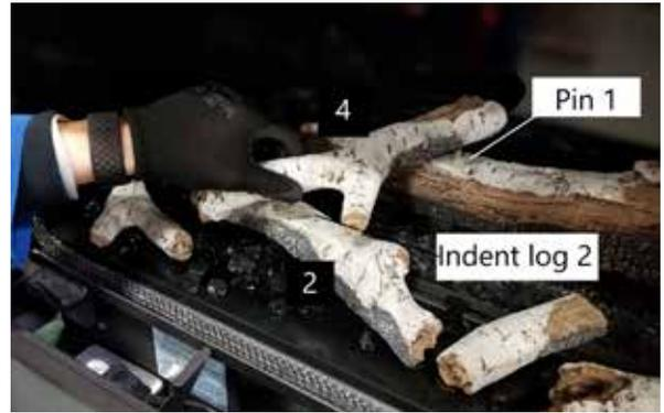
12. Place Log 5—identify the pin locator and match with the right side pin on Log 1. Rest the Log 5 on the indent in Log 3 as shown below.
