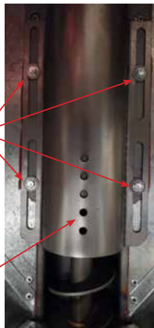
Hopper auger cover. Adjusted to accommodate larger pellets.
