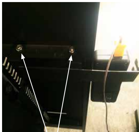
Loosen these two bolts and slide in the bracket.
