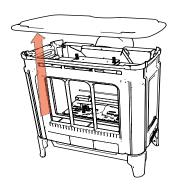
3. Loosen 2 bolts using a 7/16" (11 mm) socket and slide up light assembly bracket and place light assembly out of the way.
