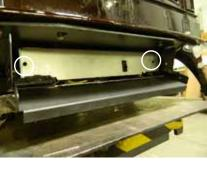
front) access panel by removing 1 screw and disconnect the NG stepper motor wires from the receiver in locations shown below.
