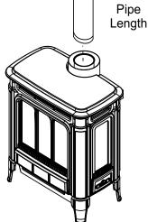
When using Rigid Vent other than Simpson Dura-Vent, 3 screws must be used to secure rigid pipe to adaptor.
