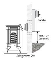
\*As specified in CSA B149.1 Installation Code. Local codes or regulations may require different clearances.
