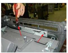
4. Remove one (1) screw to remove bulb housing.
