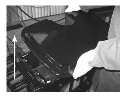
**2.** Open the two latches to remove Glass Front. Angle out and then lift, same as Cast Front.
