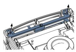
Lift light assy bracket off bolts to replace bulb
