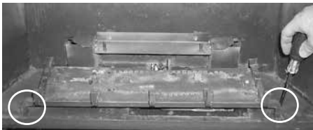
Remove the 2 screws, push Burner Assembly to the left and lift out.
