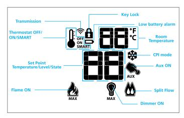
Figure 2: Transmitter LCD Display
