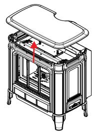
**3.** Loosen bolts securing cast front–slide light assembly bracket upward to release.
