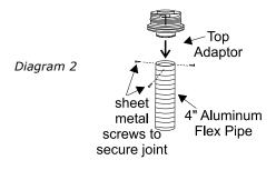
4) Pass the flex pipe down through the center of the chimney system, and center the adaptor on the top of the chimney pipe. Drill four 1/8" diameter holes through the adaptor and into the chimney top. Insure that you are in fact, drilling into the metal on the chimney. Twistlock the Termination Cap onto the Adaptor. (Diagram 3 and 4).
