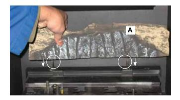
4) Place the rear log on the 2 rear log locating pins on the rear of the burner with the flat side to the back.
