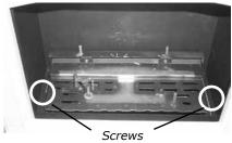
10. Remove 10 screws to remove valve tray.
