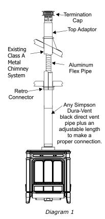
Connect the end of the flex pipe section to the underside of the Top Adaptor using 3 sheet metal screws. Diagram 2.
