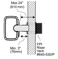
NOTE: Ensure compliance with the outside vent terminal location before cutting hole as both dimensions must be met.
