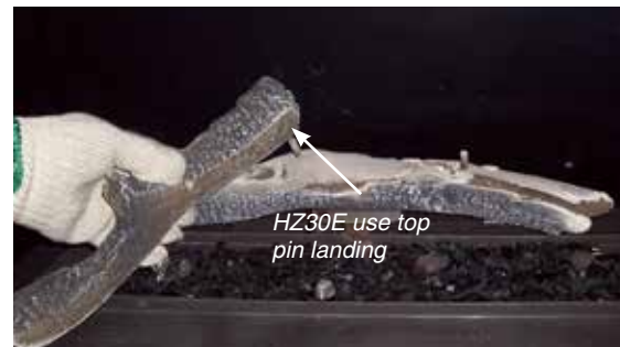
HZ30E shown - installing Log 2
