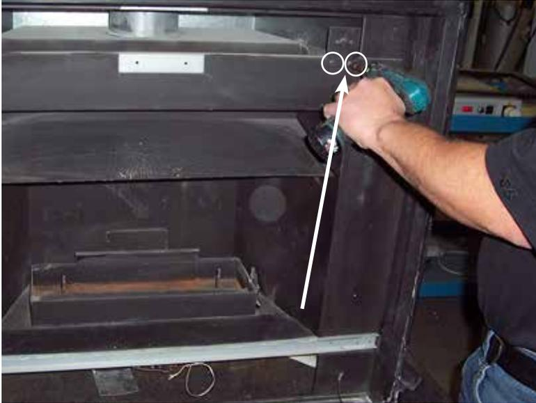
*Retirer 2 vis - retirer le support du thermodisque*
