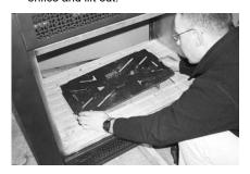
8) Remove the Side Base Brick Panels and finally the Long Base Brick Panels.
