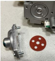
5.Install new gasket and LP regulator. Use the 2 screws provided in the kit.
