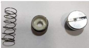
5. Install new spring and nylon screw supplied in kit. **Turn nylon screw 10 full turns and stop. Do not bottom out screw**. Gas pressure must now be checked using a manometer, refer to rating plate for exact pressures. Once completed install new red cap supplied in kit.
