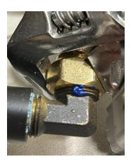
8. Remove 90 elbow containing main NG burner orifice as per below with an open end wrench & discard.
