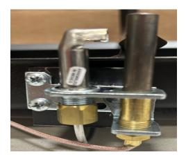
4. Remove slotted cap screw from regulator. Remove slotted nylon screw and spring. Discard all parts shown below.
