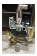
3. Replace NG orifice with supplied LP pilot orifice and reverse steps to install.
