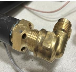
10. Reattach gas flex hose. Completed install of LP burner orifice. Test all connections for gas leaks including pilot tube disconnected in step 2.
