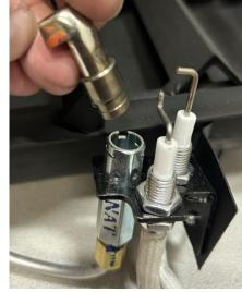
2.Locate pilot orifice screw, remove using flat head screwdriver. Replace with LP screw and reinstall.
