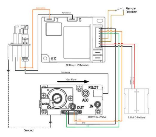
**IMPORTANT:** Ensure that there are 2 x D batteries installed as per diagram 1. The appliance will not operate without batteries in place. Ensure when batteries are in place they are polarity correct.
