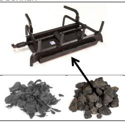
Tear or Rip embers in pieces as small as possible. Use either a comb or brush to achieve this. The smaller the piece, the better the ember glows. Spread the embers across the front burner and fill up the pan. The front burner should be completely covered. Dump lava rock around the burner covering the hearth.
