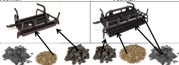
Tear or Rip embers in pieces as small as possible. Use either a comb or brush to achieve this. The smaller the piece, the better the ember glows. Pour vermiculite across the front burner. Spread the embers across the front burner and fill up the pan. Dump lava rock around the burner covering the hearth.
