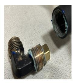
9. Apply thread sealant on LP burner orifice and install. Notice arrow on fitting showing direction of flow.
