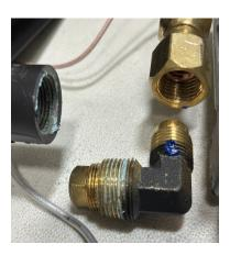
9. Apply thread sealant & install new LP orifice, note the arrow showing the flow of gas. Next, apply thread sealant to the other side of the LP orifice & install brass 90-degree elbow. Elbow should point to the front of the burner when complete. See below arrow pointing inwards toward burner.
