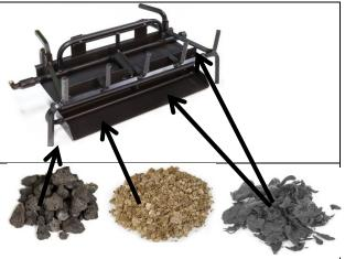
Tear or Rip embers in pieces as small as possible. Use either a comb or brush to achieve this. The smaller the piece, the better the ember glows. Pour Vermiculite along the bottom ember bed. Spread the embers across the front burner, and fill up the pan. The front burner should be completely covered. Dump lava rock around the burner covering the hearth.
