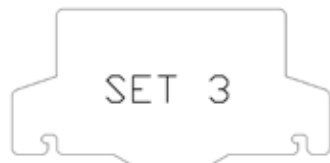
Restrictor plate for Set 3 (Part # 761-143F)
