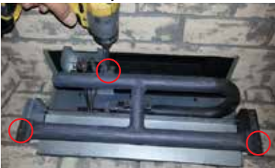
Diagram 2: Slide burner assembly to the right—then remove.
