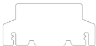
Restrictor plate for Set 1, Set 2 (Part # 761-060F)
