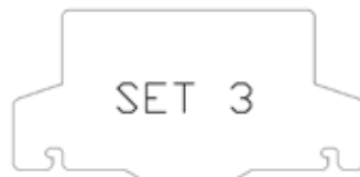
Restrictor plate for Set 3 (Part # 761-143F)
