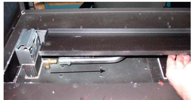
**9) Remove cover plate located in the centre of the firebox floor by removing 4 screws. Discard the cover plate and gasket - keep the screws.**
