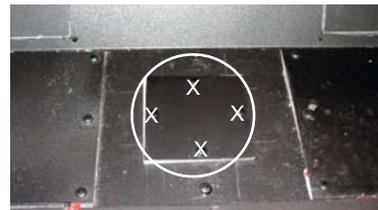
**10) Feed the plug wiring through the opening in the middle of the firebox - secure light assembly mounting plate with 4 screws (use screws from cover plate).**
