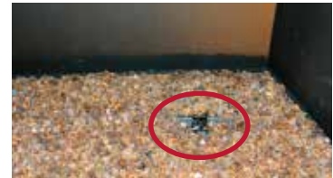
5) Ensure Crystals DO NOT block the front of the pilot hood and flame to light the burner
