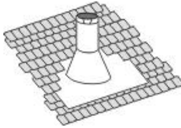
Diagram 10: The upper half of the flashing is installed under the roofing material and not nailed down until the chimney is installed. This allows for small adjustments.
