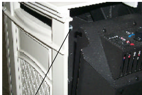
screw Lift Rear Panel off the 2 top screws
