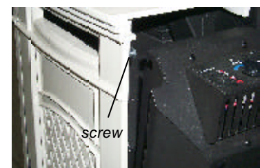
Lift Rear Panel off the 2 top screws
