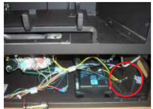
The Surefire switch is located in the right corner as shown above.
