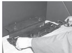
6) Remove the 2 screws, one on each side of the burner. Slide the burner to the left and then lift out.
