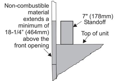
**Install Top Standoffs & Side Nailing Strips before unit is slipped into position. See the "Unit Assembly Prior to Installation" section for assembly details.**
