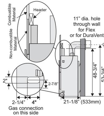
**Note:** 53-3/4" is the minimum height for both flex termination or Simpson Dura-Vent venting.
