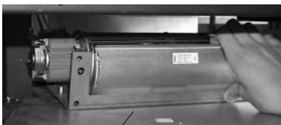
Position Fan B on mounting studs.
