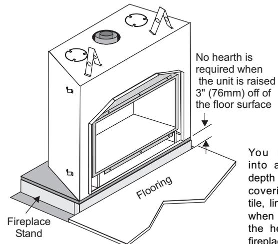
You must take into account the depth of the floor covering (carpet, tile, linoleum, etc.) when determining the height of the fireplace stand.
