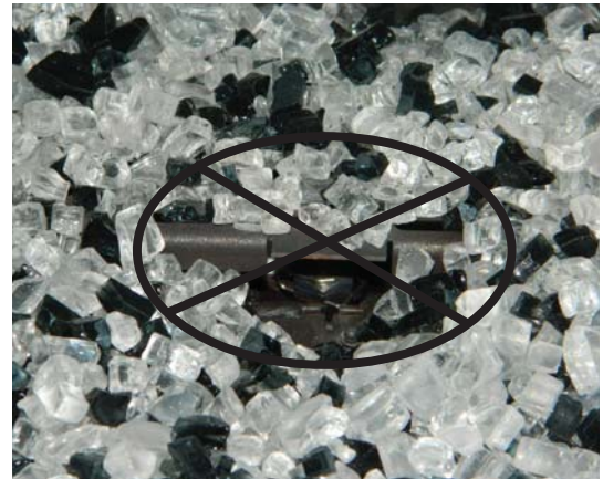
DO NOT block pilot area with glass crystals
