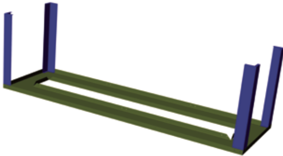
Diagram 1 - Corner supports on lower frame.
