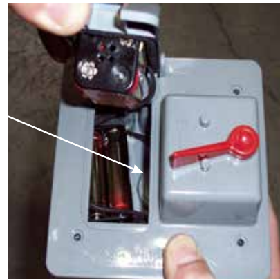
Slide 1st battery pack to the right.
