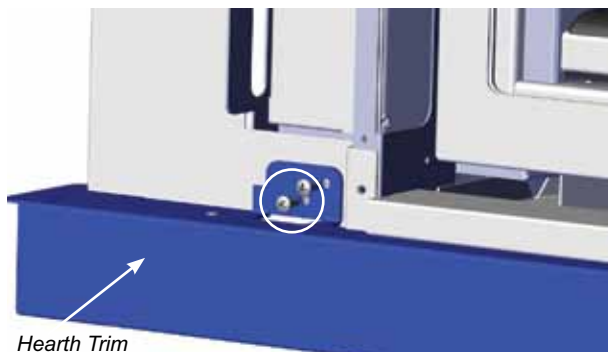
Diagram 3—Hearth Trim Secured to Backing Plate
