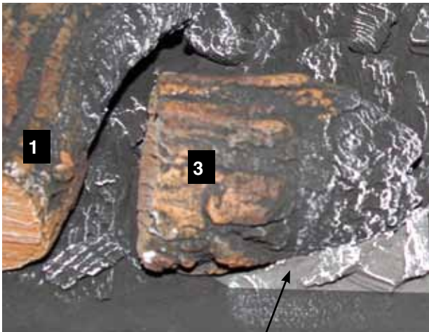
Ridge in burner tray (highlighted)
