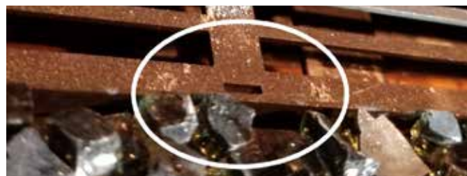
Burner covered with Fireglass and glowing wool
